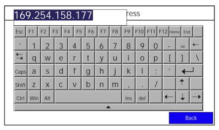
6. Repeat step 5 to enter the address for the Subnet Mask and Gateway Address.
