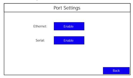
**4.** The Ethernet and Serial ports are enabled by default. Press Enable for the respective port to disable it, then press OK to confirm.
