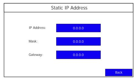
**5.** Press the blue area next to IP Address to enter an IP address in the Static IP address field.
